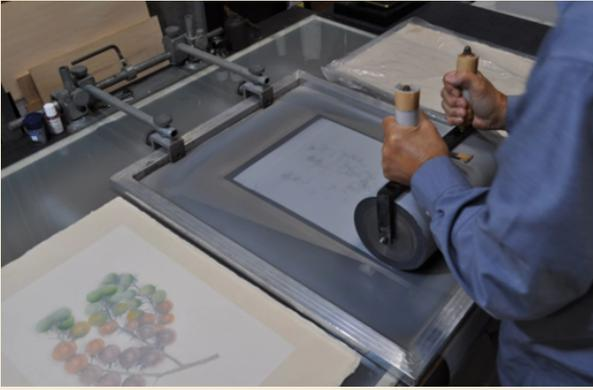
C. Pressing the ink through the stencil onto the paper with a roller as part of the silkscreen printing process
