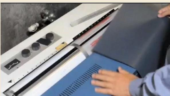
G. Using a mimeograph machine to burn holes in the vinyl film, transforming the vinyl film into a stencil based on the image from the photographic paper
